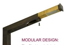
The PL-11 path light is constructed of extruded yellow brass 1" square tubing. The components that house and seal the lamp are machined to prevent corrosion from all types of elements. Stainless steel hardware. To relamp this luminaire, simply remove one screw and slide out the lamp housing.
